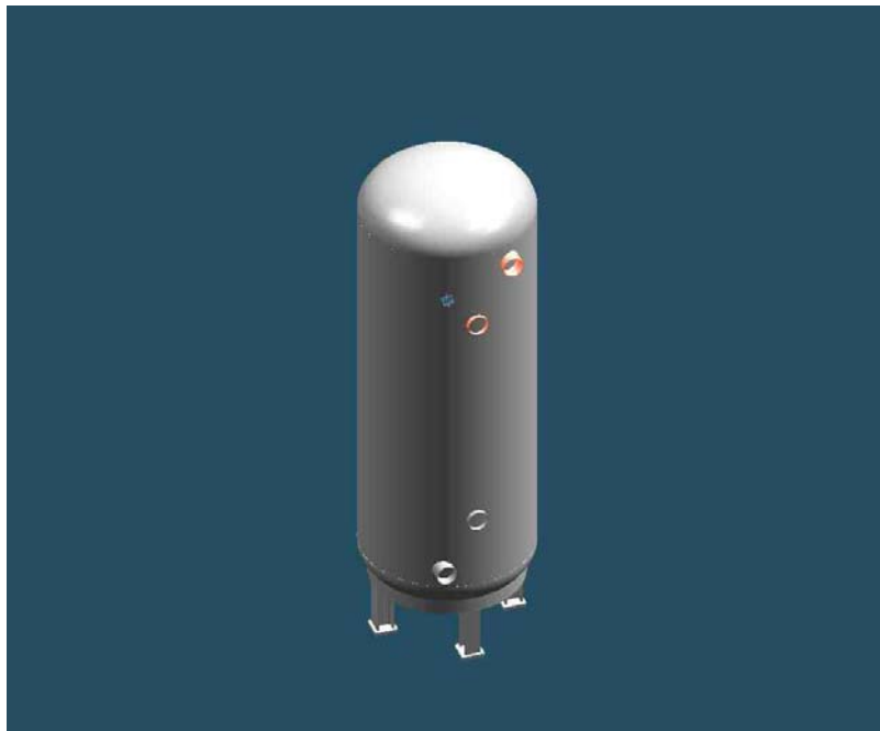
Figure C.1 – IHX unit pressure vessel
