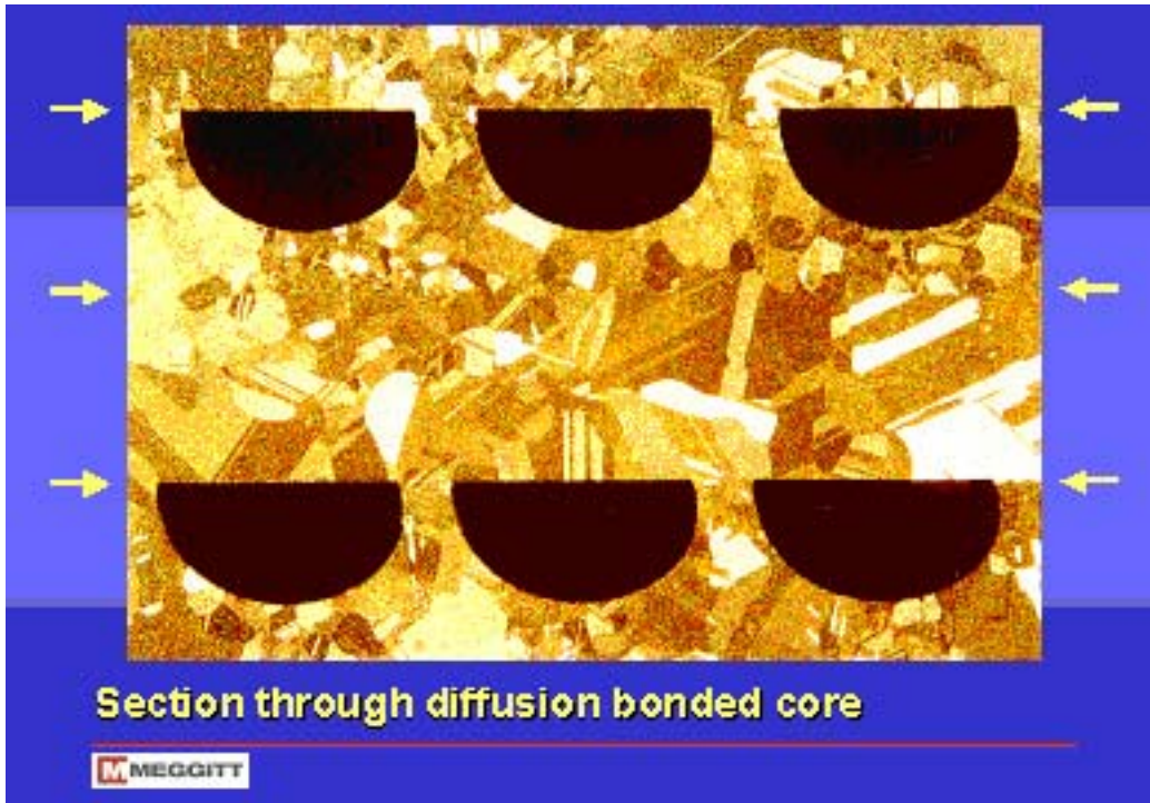
Figure 3.6 Detail of bonded printed circuit plates [7]
